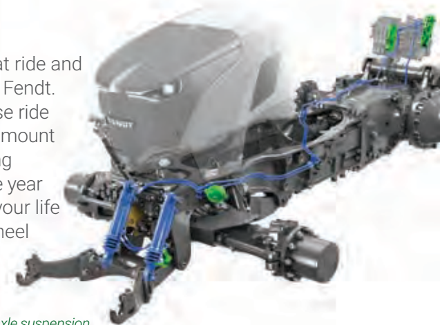
Self-leveling front-axle suspension provides a better ride and tractive ability.
