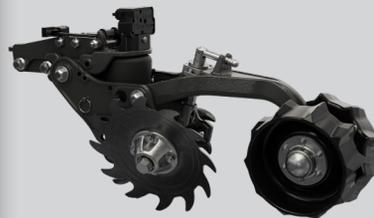
FurrowForce® from Precision Planting is an automated row-by-row control system that provides visibility to closing performance on the 20i20 display in the cab. FurrowForce uses two stages to both close the furrow and manage soil density. The first stage pinch wheels are set wider than traditional systems and move soil horizontally to remove air gaps. Following are the second-stage stitch wheels that create the proper soil density for moisture retention and optimal germination.
