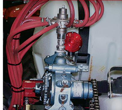
The piston pump flow divider provides optimum liquid fertilizer metering accuracy to each fertilizer opener. The application rate per acre remains constant over a wide range of planting speeds.
