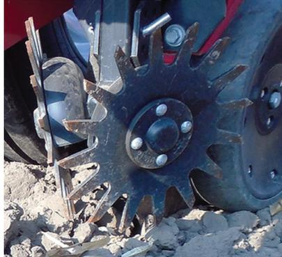
Ideal for medium- to high-residue levels, the 13 in. (330 mm) diameter pin adjust steel finger or SharkTooth wheels clear residue away from the seed opener. Adjusts in 1/4 in. (6 mm) increments.
