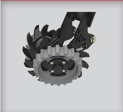
13 in. (330 mm) SharkTooth or finger wheels and depth bands provide aggressive residue movement from the path of the row unit. The unit-mounted residue wheels float over the surface, and the depth bands assure the right depth of operation.
