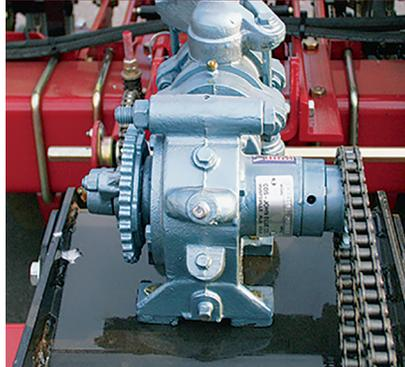
The variable-stroke, double-acting, single- or double-piston metering pump dispenses a consistent flow of liquid fertilizer. All internal parts that come in contact with the fertilizer are stainless steel.
