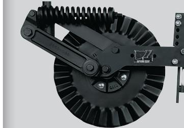
Designed for no-till, minimum-till and conventional tillage operations, this single disc fertilizer opener/liquid injector features a spring-mounted tine injector nozzle for liquid fertilizer application. Liquid fertilizer is placed in the soil without the use of a knife, providing plug-free operation.
