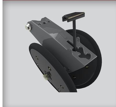
Improve seed-to-soil contact in heavier soil and moderate no-till conditions. Adjust wheels by offsetting them or changing width from 1.25 to 2.88 in. (32 to 73 mm) for improved performance at various seed depth and soil conditions. Adjustable down pressure: 50 to 133 lbs. (23-133 kg.).
