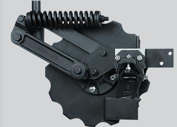
Designed for no-till and minimum-till applications, this single-disc fertilizer opener features an austempered side profile knife to place fertilizer up to 4 in. (102 mm) deep, providing effective placement of fertilizer with minimal adjustment.
