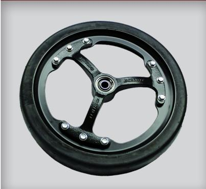
A gauge wheel deduction option is available, permitting the exclusion of the traditional 4.5 in. (114 mm) factory-installed gauge wheels. Several popular gauge wheel styles and widths are available for field installation. Choose the solid or spoked wheels in 3 in. (76 mm) or 4.5 in. (114 mm) widths, as well as gauge wheel scrapers.
