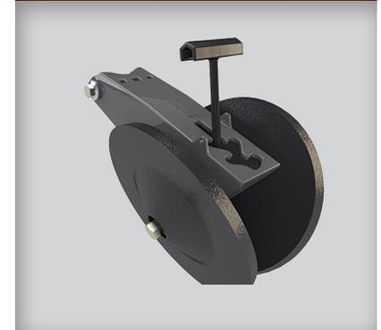
Great for closing the toughest seed trench. Recommended for tough no-till conditions. Adjust wheels by offsetting or changing width for improved performance in high-residue and no-till conditions. Adjustable down pressure: 115 to 310 lbs. (52-141 kg.).
