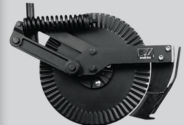
Designed for no-till planting conditions, this 17 in. (432 mm) disc and knife work well in firm, no-till soil that has residue on the soil surface. The disc cuts residue at the soil surface, and the trailing knife places the fertilizer with minimum soil disturbance.
