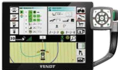
The Variotronic headland management saves all the procedures when performing a turning maneuver. Variotronic automatically triggers the sequences precisely at the right place.
