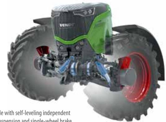
Front axle with self-leveling independent wheel suspension and single-wheel brake.
