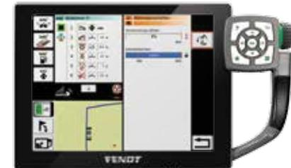
The coolant level and degree of air filter contamination are shown in the Varioterminale™.
