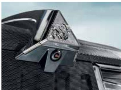
Practical for front-mounted implements, the new camera integrated in the hood captures the view to the lower links and transmits the image to the Varioterminal.
