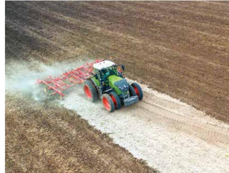
Thanks to the TMS and automatic maximum output control 2.0, the tractor optimally adapts the engine speed to the driving speed.
