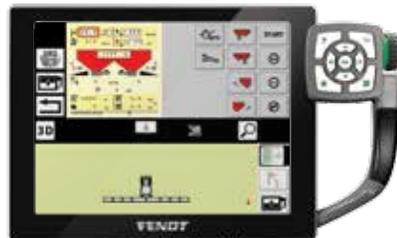
You can control ISOBUS-capable implements via Variotronic implement control directly via the joystick or Varioterminal.
