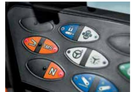
Tried and tested Fendt operating logic arranges all functions simply and clearly on the backlit membrane keypad.
