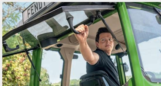
A special feature of the Fendt 200 Vario is the vertical handle on the rear window, which lets you open and close the window from the comfort of your seat.
