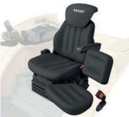
The comfort seat, with suspension and a mechanical lumbar support, offers excellent seating comfort. The instructor seat is cushioned and can be pivoted upwards to save space, if required.
