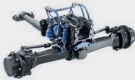
The integrated self-levelling system of the front axle suspension ensures consistent working and driving comfort at any load. The locking function for precise implement guidance in front loader mode, for example when loading pallets.
