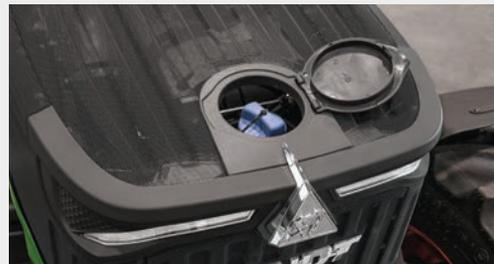
The large diesel tank with 33 gal (125 L) of diesel on the A-pillar ensures long range. Then there is the 4.2 gal (16 L) DEF tank at the front on the hood head. Work longer without refuelling.
