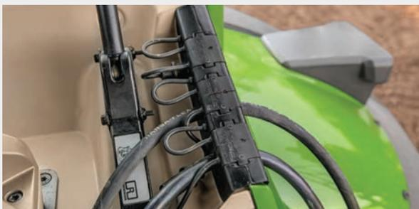
Fendt offers a clever solution for cables that run from the rear of the tractor into the cab. Cables can be guided through the lead-through, no matter what kind of cross section they have. The rear window can be closed, so dust, dirt, water and noise stay outside.
