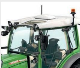
The Fendt Guide receiver is exceptionally well protected and fully integrated into the roof design. Without overhanging parts or externally guided cables, the technology is particularly well protected against hanging branches but also theft.
